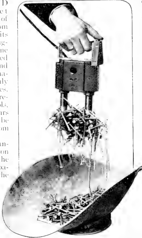
Where large quantities of brass and iron filings accumulate this magnet will be found invaluable for separating them
